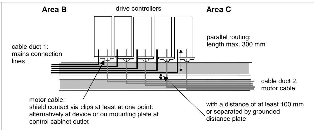
Fig. 7-23: Option 1: separate routing of motor cable and mains connection lines via 2 cable ducts
